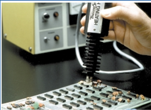
ThermoSpot® Systems for testing and fault isolation of individual components at precise hot and cold temperature at the tester socket or on a printed circuit board.
