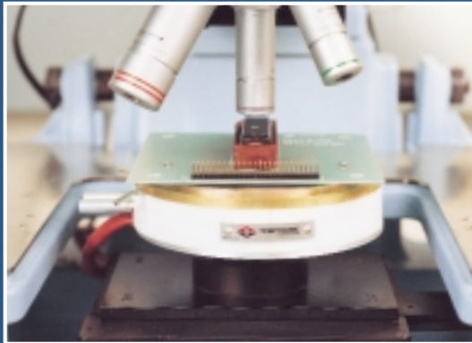
ThermoSocket® Systems for testing and locating micron size defects on chips in minutes, even at 30 microwatt power levels.
