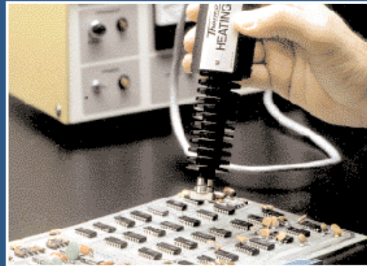
ThermoSpot® Systems for testing and fault isolation of individual components at precise hot and cold temperature at the tester socket or on a printed circuit board.
